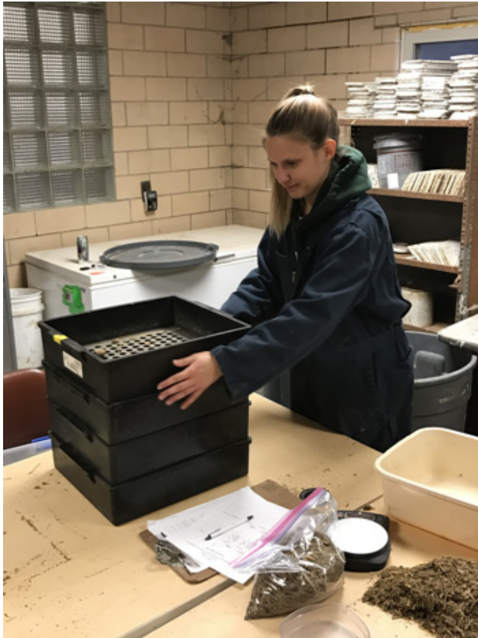
Figure 1. University of Illinois student performing the Penn State Shaker Box test on a TMR sample.
